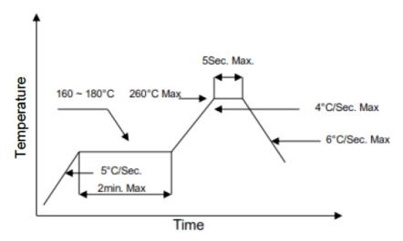
Note: Reflow soldering can be operated only one time. During the temperature ramp-up, no forces may be exerted on the LD which would deform or damage them. After soldering is completed, please do not process until the product temperature ramps down to room temperature.
