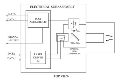
**Transmitter and Receiver Optical Sub-assembly Section** - A 1570 nm InGaAsP laser and an InGaAs PIN photodiode integrate with an WDM filter to form a bi-directional single fiber optical subassembly (OSA). The laser of OSA is driven by a LD driver IC which converts differential input LVPECL logic signals into an analog laser driving current. The photodiode of OSA is connected to a circuit providing post-amplification quantization, and optical signal detection.
