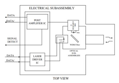
**Transmitter and Receiver Optical Sub-assembly Section** - A 1570 nm InGaAsP laser and an InGaAs PIN photodiode integrate with an WDM filter to form a bi-directional single fiber optical subassembly (OSA). The laser of OSA is driven by a LD driver IC which converts differential input LVPECL logic signals into an analog laser driving current. The photodiode of OSA is connected to a circuit providing post-amplification quantization, and optical signal detection.
