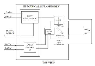
**Transmitter and Receiver Optical Sub-assembly Section** - A 1510 nm InGaAsP laser and an InGaAs PIN photodiode integrate with an WDM filter to form a bi-directional single fiber optical subassembly (OSA). The laser of OSA is driven by a LD driver IC which converts differential input LVPECL logic signals into an analog laser driving current. The photodiode of OSA is connected to a circuit providing post-amplification quantization, and optical signal detection.
