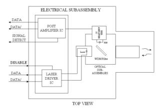
Transmitter and Receiver Optical Sub-assembly Section - A 1550 nm InGaAsP laser and an InGaAs PIN photodiode integrate with an WDM filter to form a bi-directional single fiber optical subassembly (OSA). The laser of OSA is driven by a LD driver IC which converts differential input LVPECL logic signals into an analog laser driving current. The photodiode of OSA is connected to a circuit providing post-amplification quantization, and optical signal detection.
