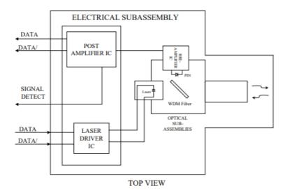
**Transmitter and Receiver Optical Sub-assembly Section** - A 1550 nm InGaAsP laser and an InGaAs PIN photodiode integrate with an WDM filter to form a bi-directional single fiber optical subassembly (OSA). The laser of OSA is driven by a LD driver IC which converts differential input LVPECL logic signals into an analog laser driving current. The photodiode of OSA is connected to a circuit providing post-amplification quantization, and optical signal detection.
