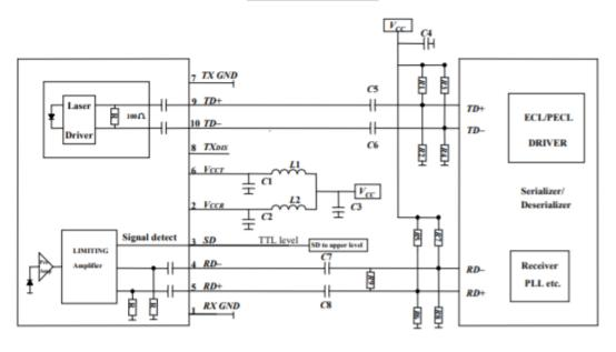
C1/C2/C4/C5/C6/C7/C8 = 100 nF  $C3 = 4.7 \ \mu\text{F}$   $L1/L2 = 1\ \mu\text{H}$ R1/R2/R3/R4/R5/R6/R7/R8/R9 Depend on SerDes
