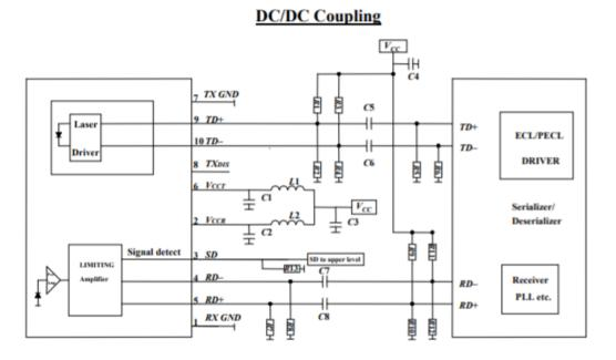
C1/C2/C4/C5/C6/C7/C8 = 100 nF $R1/R3 = 82\Omega$  $R13 = 180 \Omega (PECL)$
