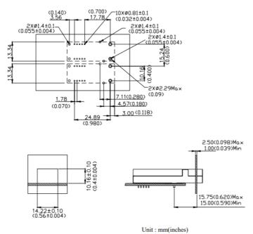
This transceiver is compatible with industry standard wave or hand solder processes. After wash process, all moisture must be completely removed from the module. The transceiver is supplied with a process plug to prevent contamination during wave solder and aqueous rinse as well as during handling, shipping or storage.
