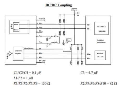
In order to get proper functionality, a recommended circuit is provided in above recommended circuit schematic. When designing the circuit interface, there are a few fundamental guidelines to follow.
