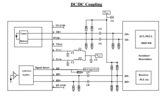
C1/C2/C4/C5/C6/C7/C8 = 100 nF $C3 = 4.7 \ \mu\text{F}$  $L1/L2 = 1 \ \mu\text{H}$  $R1/R3 = 82\Omega$  $R2/R4 = 130 \ \Omega$  $R7/R8 = 130 \ \Omega$  $R13 = 180 \ \Omega$  (PECL)R5/R6/R9/R10/R11/R12 Depend on SerDes
