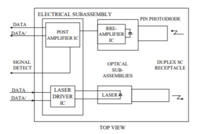
**Transmitter Section** - The transmitter section consists of a 1550 nm InGaAsP in an eye safe optical subassembly (OSA) which mates to the fiber cable. The laser OSA is driven by a LD driver IC which converts differential input LVPECL logic signals into an analog laser driving current.
