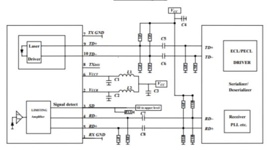
C1/C2/C4/C5/C6/C7/C8 = 100 nF $R1/R3 = 82\Omega$   $C3 = 4.7 \mu F$  $R2/R4 = 130 \Omega$   $L1/L2 = 1 \mu H$  $R7/R8 = 130 \Omega$
