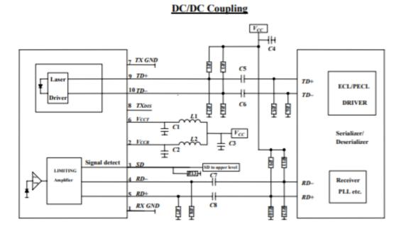
$\begin{array}{ll} C1/C2/C4/C5/C6/C7/C8 = 100 \text{ nF} & C3 = 4.7 \ \mu\text{F} & L1/L2 = 1 \ \mu\text{H} \\ R1/R3 = 82\Omega & R2/R4 = 130 \ \Omega & R7/R8 = 130 \ \Omega \\ R13 = 180 \ \Omega & (\text{PECL}) & R5/R6/R9/R10/R11/R12 \text{ Depend on SerDes} \end{array}$
