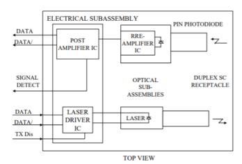
**Transmitter Section** - The transmitter section consists of a 1310 nm InGaAsP laser in an eye safe optical subassembly (OSA) which mates to the fiber cable. The laser OSA is driven by a LD driver IC which converts differential input LVPECL logic signals into an analog laser driving current.
