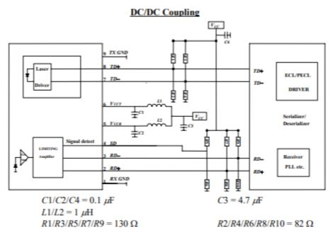
In order to get proper functionality, a recommended circuit is provided in above recommended circuit schematic. When designing the circuit interface, there are a few fundamental guidelines to follow.
