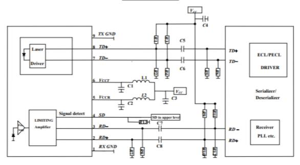
C1/C2/C4/C5/C6/C7/C8 = 100 nF $R1/R3 = 82\Omega$ ,  $C3 = 4.7 \mu F$  $R2/R4 = 130 \Omega$   $L1/L2 = 1 \mu H$  $R7/R8 = 180 \Omega$
