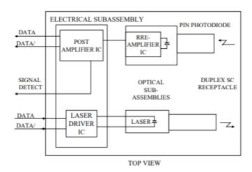
**Transmitter Section** - The transmitter section consists of a 1310 nm InGaAsP laser in an eye safe optical subassembly (OSA) which mates to the fiber cable. The laser OSA is driven by a LD driver IC which converts differential input LVPECL/PECL logic signals into an analog laser driving current.
