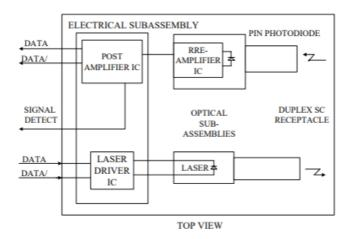
**Transmitter Section** - The transmitter section consists of a 1310nm InGaAsP in an optical subassembly (OSA) which mates to the fiber cable. The laser OSA is driven by a LD driver IC which converts differential input LVPECL logic signals into an analog laser driving current.
