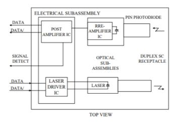
**Transmitter Section** - The transmitter section consists of a 1310nm InGaAsP in an optical subassembly (OSA) which mates to the fiber cable. The laser OSA is driven by a LD driver IC which converts differential input LVPECL logic signals into an analog laser driving current.
